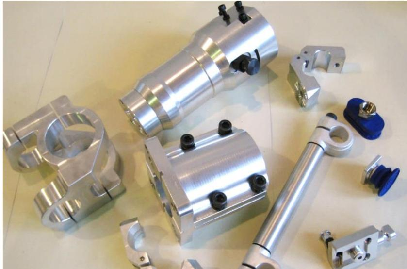
**EOAT** – End of arm tooling or end effectors are devices of the robot's arm that enable variety of solutions on robotized systems in all industrial branches.
